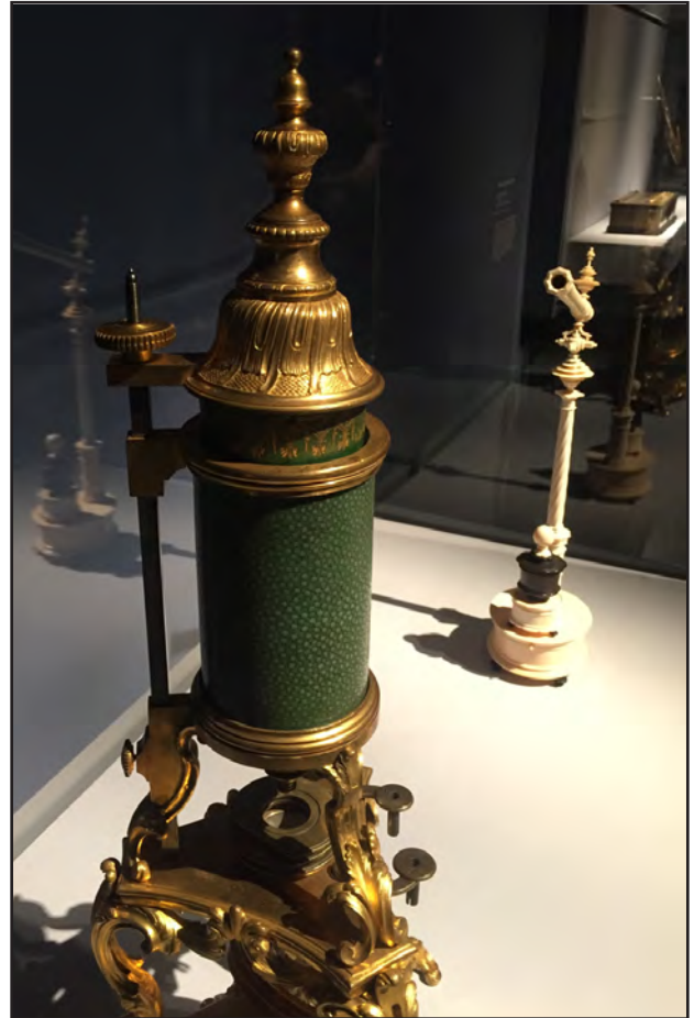
Above the focusing rack can be seen to the left of the body tube. Below the stage mount and the armature, perhaps for stage forceps.
