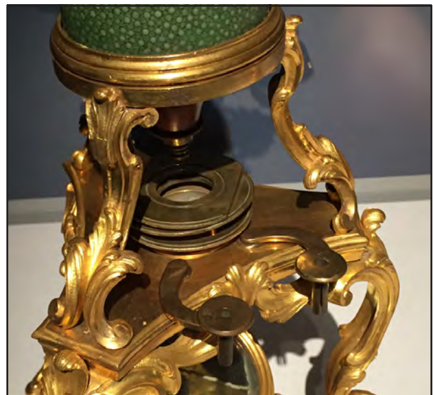
Above the focusing rack can be seen to the left of the body tube. Below the stage mount and the armature, perhaps for stage forceps.
