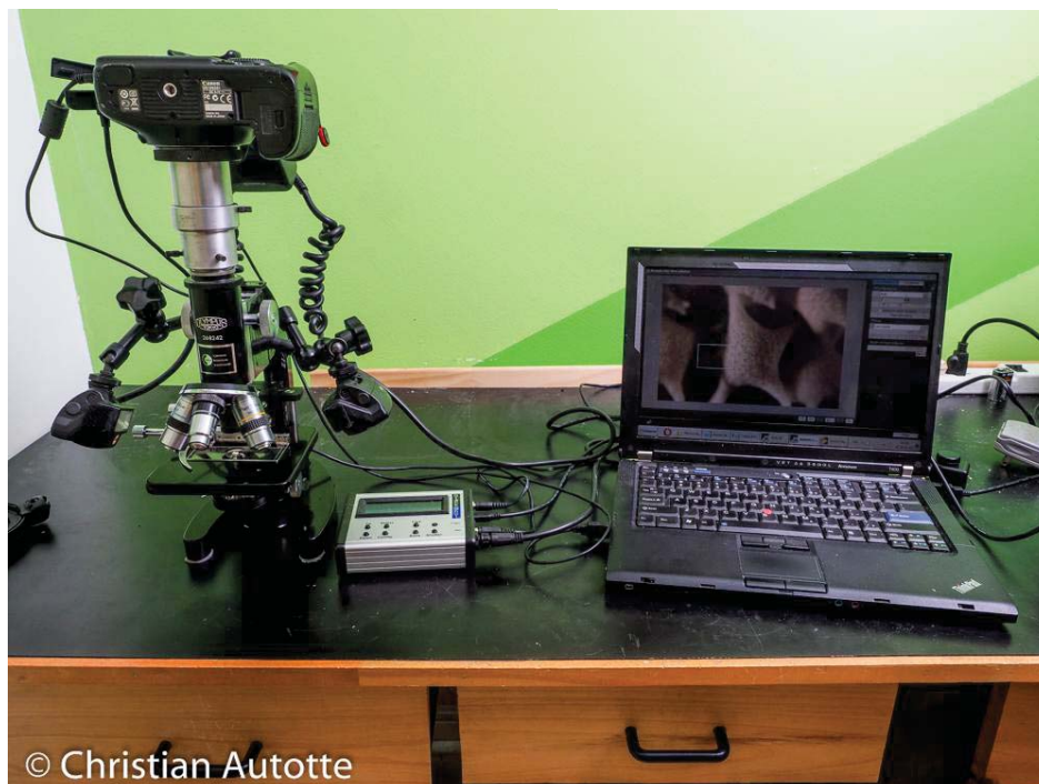
The stacking microscope in action, controlled by Zerene Stacker through a laptop computer
