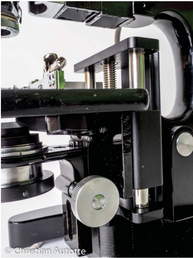
Details showing the rail with the stage and condenser
