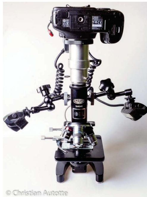
A pair of "twin flash" on articulated arms
