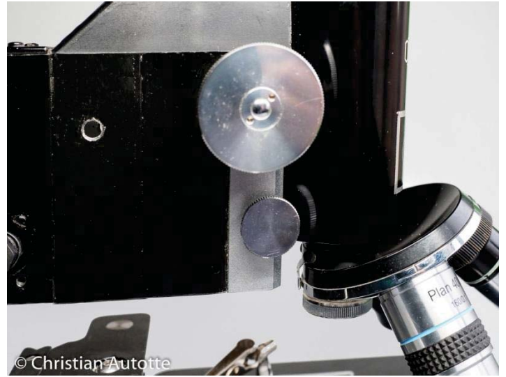
An extra screw added under the coarse focus to lock it in place
