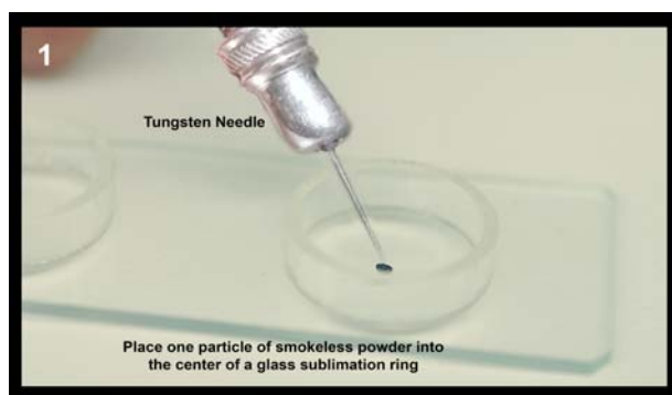
Figure 1 - One particle or wafer of smokeless is placed with a sharp tungsten needle on the surface of a glass microscope slide within the center of a glass ring.
