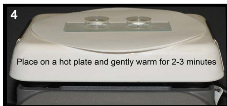
Figure 4 - The slide containing the blank (left) and the suspected particle (right) are placed on a hot plate and gently warmed for a few minutes.
