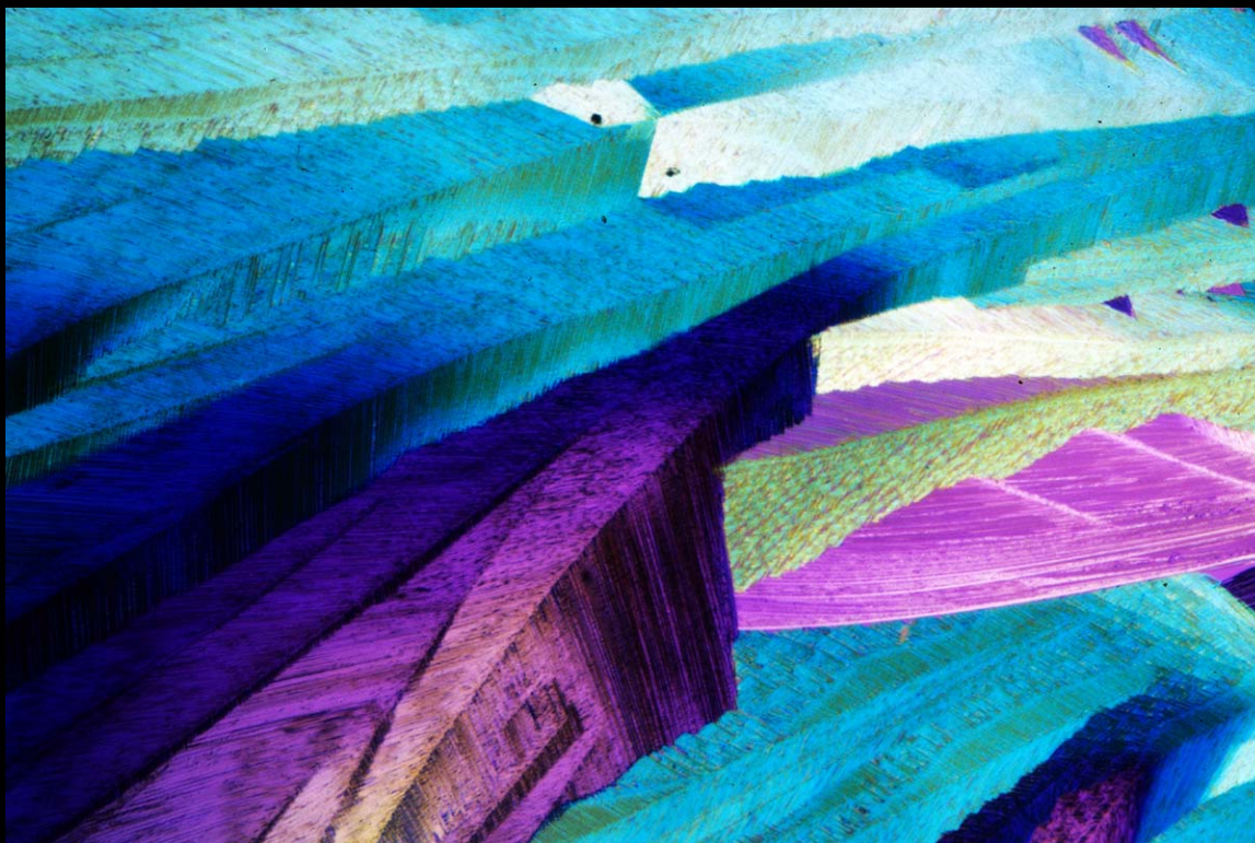
Butylated Hydroxy Toluol from melt (BHT), 50x (P1053126)a6x4x200 Preparation and polarixed-light photomicrograph by Mel Pollinger
