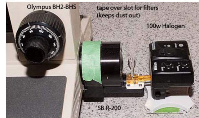
Fig. 2. Olympus lamp box removed, flash used to make the image
