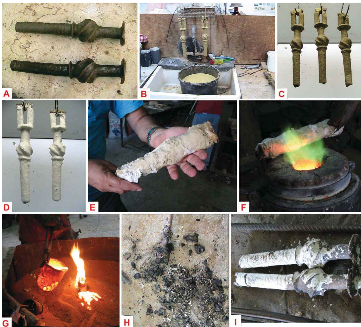
Figure 4a–i. Modern simulation of the casting process of the Chalcolithic standard shown in fig. 3 (refer to the text for details). Photographs and graphics by Y. Goren.
