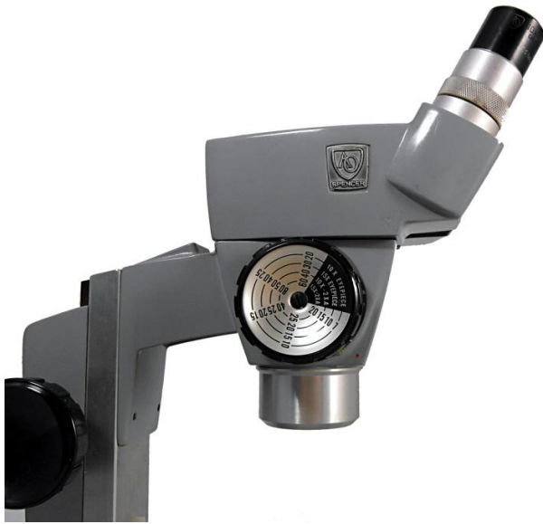
Figure 13. Viewing tubes facing away from column support
