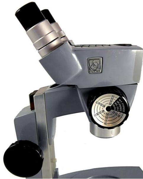
Figure 14. Viewing tubes facing toward column support
