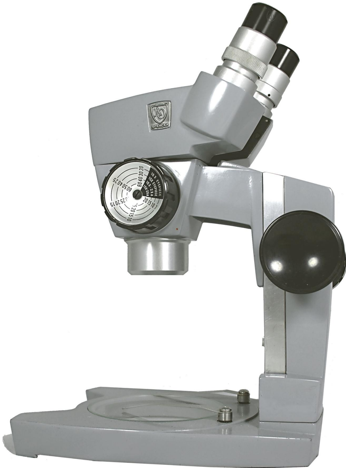
Figure 8. AO Cycloptic model for reflected light, with Magni-Changer "M" (Kreindler, September 2012)
