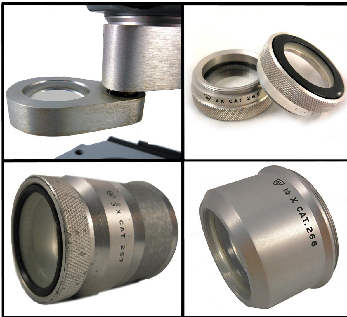
Figure 26. Cycloptic Auxiliary lenses (a) 2X Swing-out, (b) 2X fixed examples, (c) 2/3X mounted (d) 0.5X,
