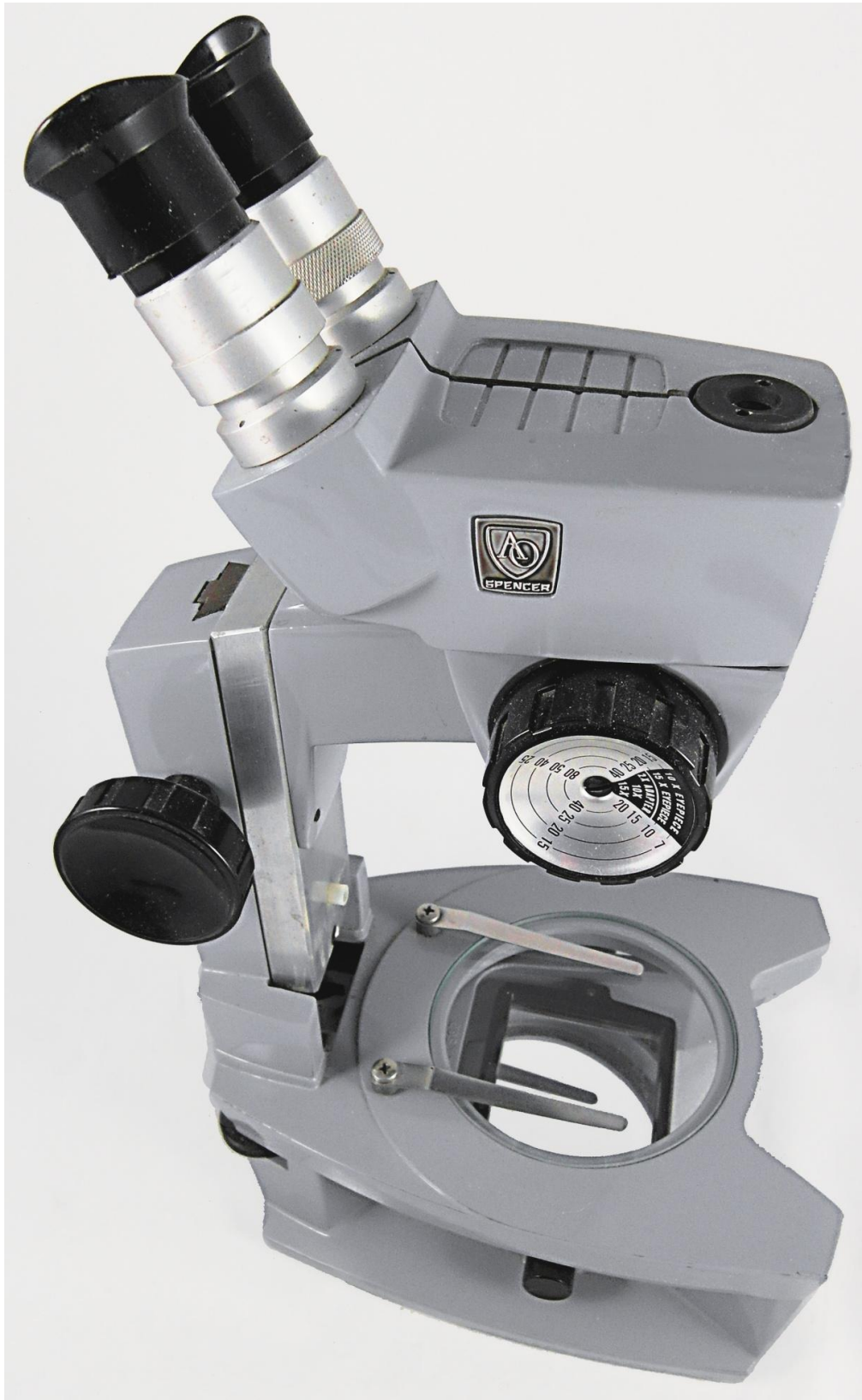
Figure 21. Cycloptic with Transilluminating Substage Base installed
