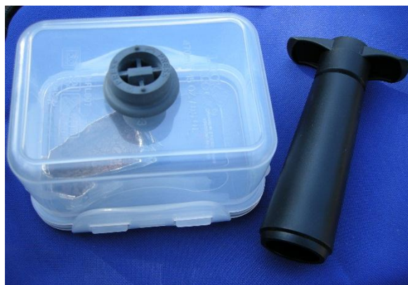
Figure 11: Improvised vacuum desiccator for sample impregnation made of a microwave lunch box and a wine-stopper pump. Notice the sample in the aluminum foil mold inside the box
