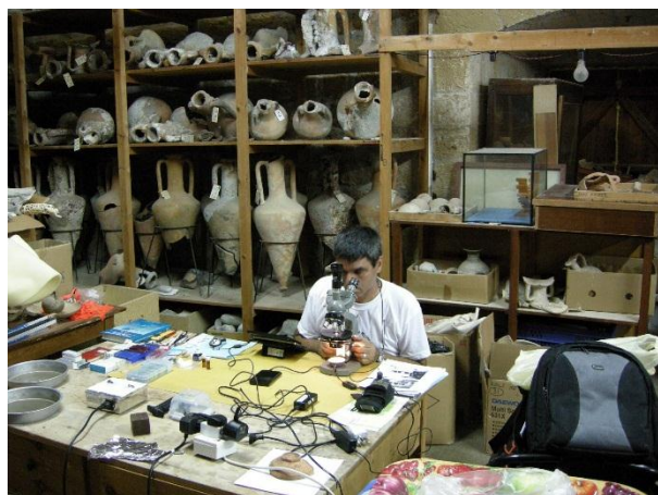
Figure 2: On site petrographic examination of pottery vessels from the fifth-century BC Kyrenia shipwreck at the Ship Museum in Kyrenia (Northern Cyprus). Some of the amphorae from the ship are seen behind the microscopist. The portable thin section laboratory was brought in the backpack seen at the lower right corner, enabled the preparation and examination of approximately 100 thin sections within a few days
