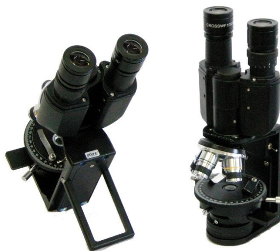
Figure 17: The commercial version of the Goren portable petrographic microscope, now available from MRC Ltd. Laboratory Equipment . The microscope offers laboratory-level optical quality, ergonomics, and performance but with self-sustained power in small, portable dimensions. A biological version with X-Y mechanical stage, 100X oil objective, and optional phase-contrast is also available in this format
