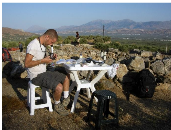
Figure 4: Operation of on-site micromorphological laboratory for the preliminary examination of small sediment samples at the Minoan site of Koumasa , Crete, summer 2012. The micromorphologist is using an early version of the Goren portable petrographic microscope to examine a sample
