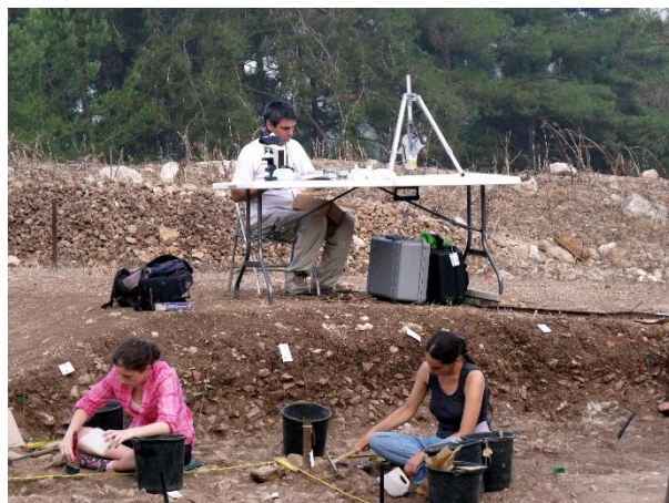
Figure 3: The operation of an on-site petrographic laboratory at the Pre-Pottery Neolithic B (about 9000 years old) site of Kfar HaHoresh , near Nazareth, Israel, in 2010. The laboratory includes a microscope, equipment for the preparation of quick petrographic thin sections, and portable XRF (on the tripod) for ad-hoc elemental analysis
