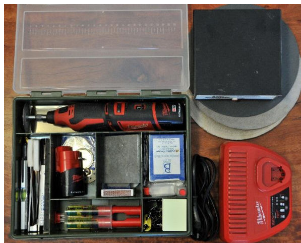
Figure 9: The portable thin-section laboratory in packed position (the scale is indicated by the cm ruler on the organizer cover). The three unpacked items on the right side are a battery charger for the rotary tool, mini hotplate, and three metallographic grinding pads.
