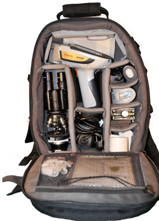
Figure 5: My backpack for flights to overseas field projects. At the top is the portable XRF, whose accessories are spread over the other compartments. The MRC® Goren portable microscope (petrographic version) is seen on the left side of the pack. The front compartment (open in the photo) contains a laptop and personal items (wallet, passport, etc.). Other equipment is packed in the checked-in suitcase ( Figure 9 )
