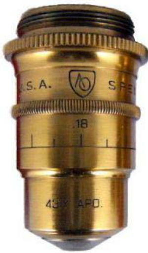
Figure 3. AO high N.A. 0.95 APO Objective
