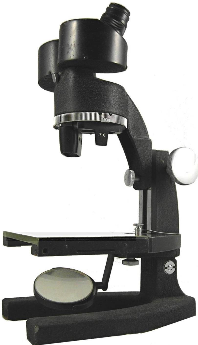
Figure 35. AO Model 25 in Black, with thumb screw height adjustment clearly visible, and with AO Number 24 detachable horseshoe base unit and mirror. If this base were detached, this would be an AO Series 26 stereomicroscope
