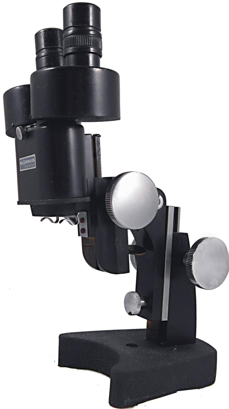
Figure 36A. AO Model 27, with 90 degree rotation around vertical axis. c. 1952
