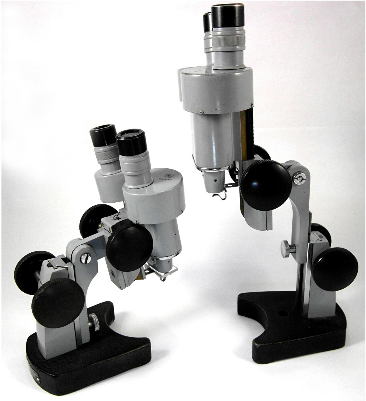
Figure 36B. AO Model 27s in gray showing the value of dual adjusting knobs for examining either small or large objects.
