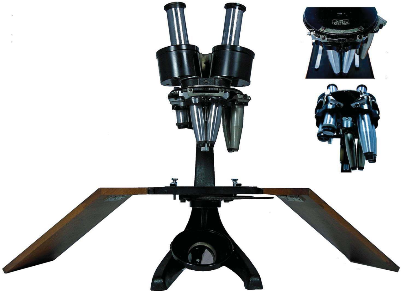
Figure 43. Zeiss 'Double tube X with revolving nosepiece', c. 1935.
