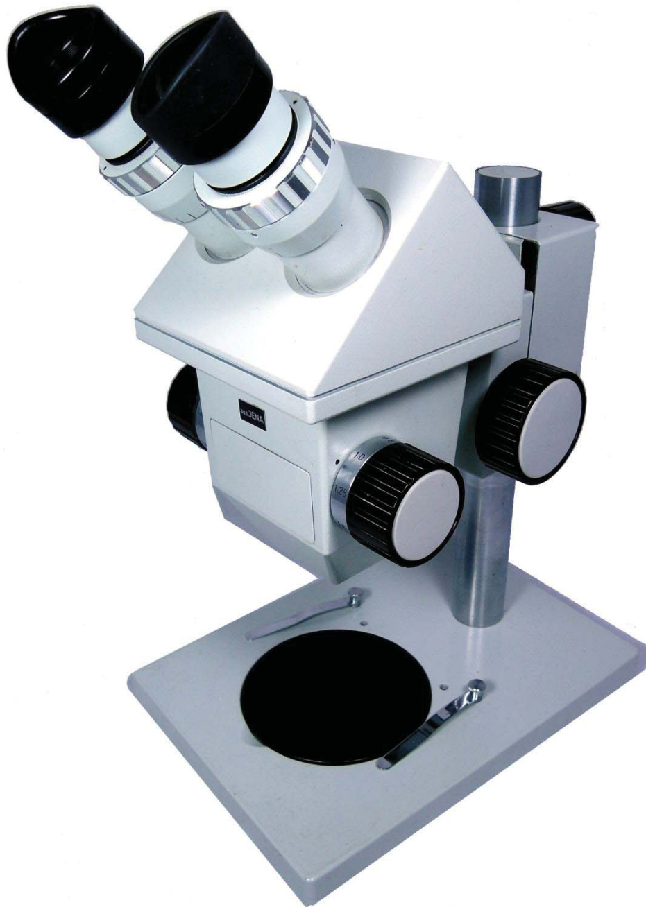
Figure 47. An aus Jena Greenough GSZ stereo microscope c. 1984 (The hard eyecup on the left eyepiece is original.)
