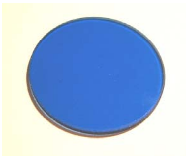
Blue Optical Glass 31.8mm diameter, and 1.33mm thick
