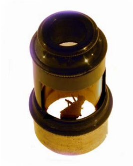
Live-chamber microscope, with beetle.
