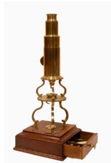
Culpeper type microscope (ca 1800), with circular stage, "fish plate" mirror, ivory and wood sample slides in drawer.
