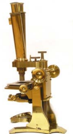
Bi-ocular microscope (ca 1860-1880) sold by Baker of London, who was an agent for Grundlach in Berlin. The scope came with an additional single tube (not shown) for monocular viewing.
